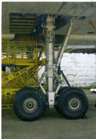
During late October, Concorde G-BBDG was put back on to its undercarriage units.
